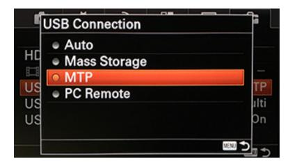
You need to re-plug and unplug USB when you switch between "Computer Remote" mode and "MTP" mode. To check full features supported by Sony cameras, please refer to <u>http://www.cam-fi.</u> <u>com/en/spec\_camera\_list.html</u>
